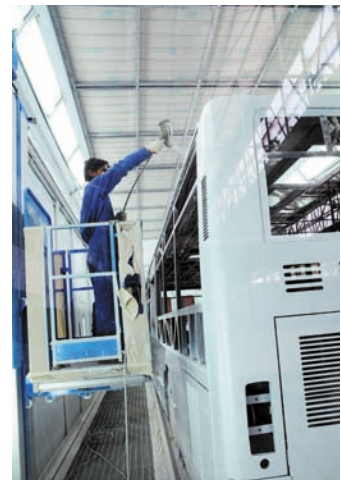
Spray painting using man-lifts
