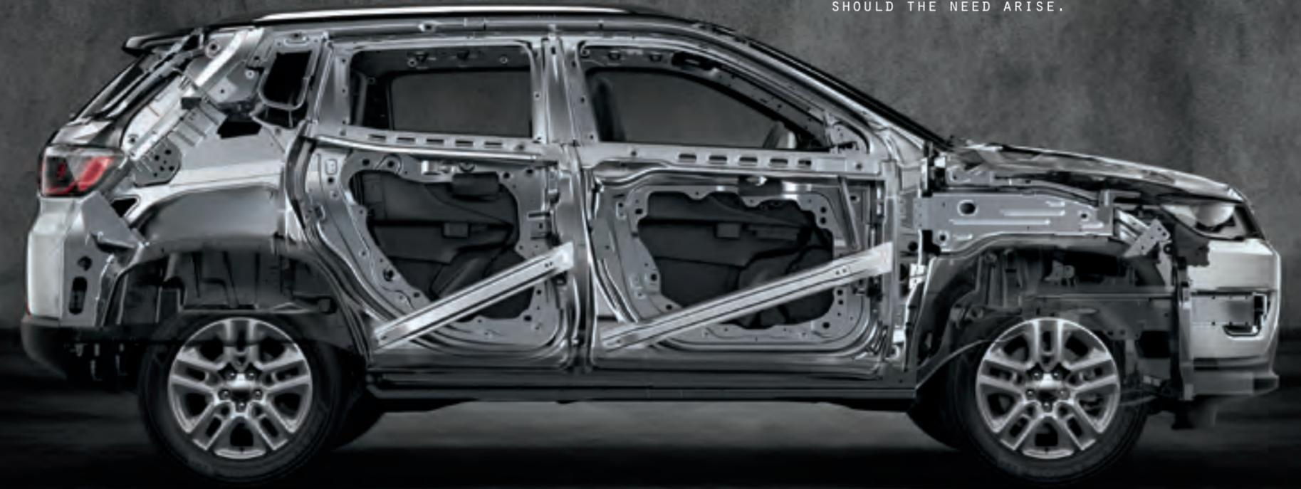
**CHASSIS STRENGTH** COMPASS DELIVERS EXCEPTIONAL PEACE OF MIND WITH A HERO'S HEART — A STRONG UNIBODY STRUCTURE IS ENGINEERED WITH APPROXIMATELY 70% HOT-STAMPED STEEL.
