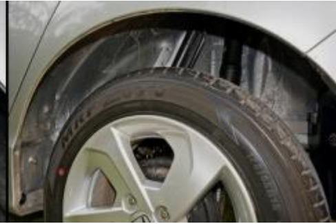
Partial cladding in Rear
