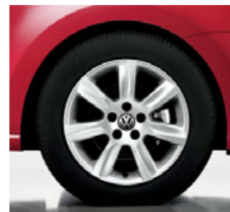
'Castille' 6J x 15 alloy wheels with 185/60 R15 tyres and anti-theft wheel bolts add a contemporary finishing touch to the exterior. Standard on SE models.
