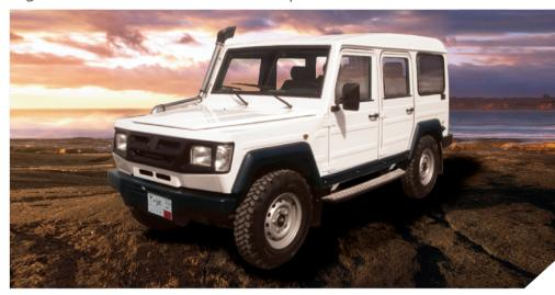
Five sided armoring of passenger compartment to provide protection against 7.62 x 51, M80 NATO Ball ammunition (CEN protection level B6).
