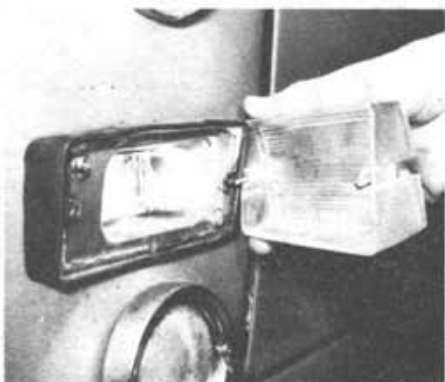
14.21 Typical back-up light (FJ 55 model)
