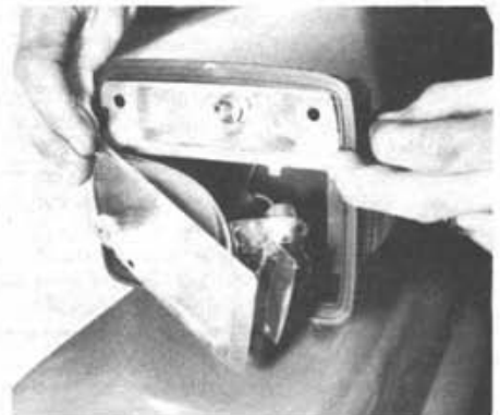
14.11b Typical arrangement for the front turn signal and sidelights (FJ 55 models)
