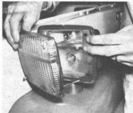
14.11a Typical arrangement for the front turn signal and sidelights (FJ 55 models)
