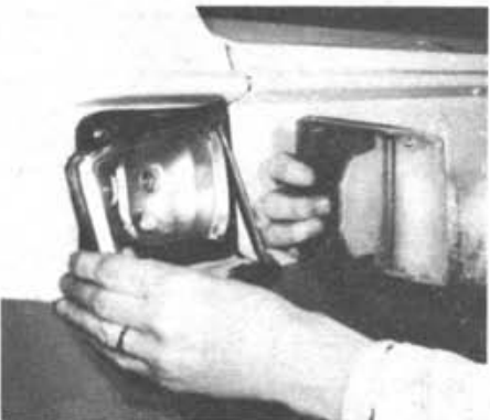
14.16a, 14.16b Typical arrangement for rear combination lamp (FJ55 models - the rear lamp bulb is missing on some models to comply with lighting regulations - see photo 14.17)
