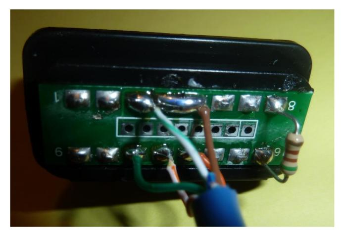
Large picture of all the connections on the OBD2 connector side. I always add additional solder to the connections after initially connecting them to be sure there's no way they will disconnect from everyday use. All you need to do now is use your multimeter to make sure you have good continuity in the wires between the OBD2 connector and RJ-45; and that the resistor is registering the correct ohm reading. See that was easy!
