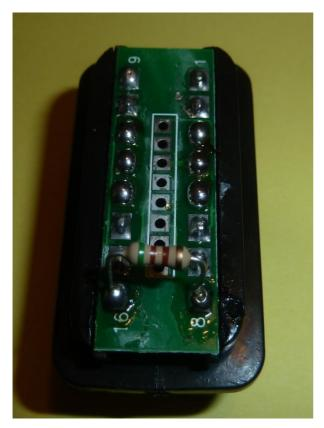
On to the OBD2 connector now. This is where the bulk of your soldering will be. You shouldn't worry about your soldering skills because no one else is going to see your work. That and its going to be covered by the casing of the OBD2 connector.
