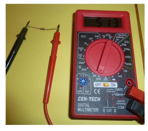
First I test the resistor to make sure it doesn't fluctuate all over the place. So long as it sits stable between 506 and 560 ohms you are set.
