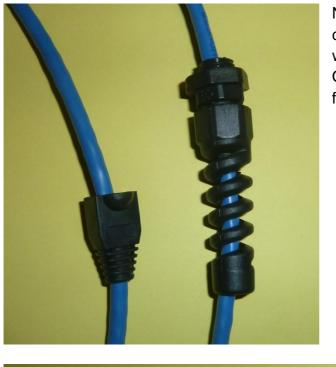
Next put on the RJ-45 boot and OBD2 connector cable protector. You don't want to crimp the RJ-45 or solder your OBD2 connector only to find out you forgot to put these on the cable first.
