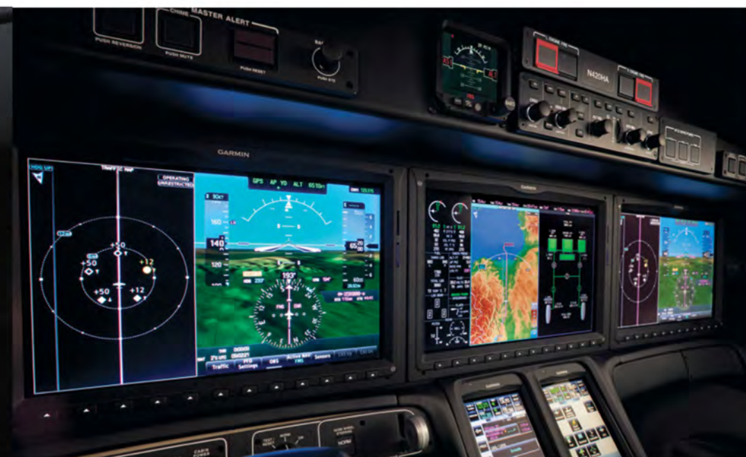
40/60 display format on the Primary Flight Displays enables maximum functional use of display space with easy visual scan for every phase of flight
