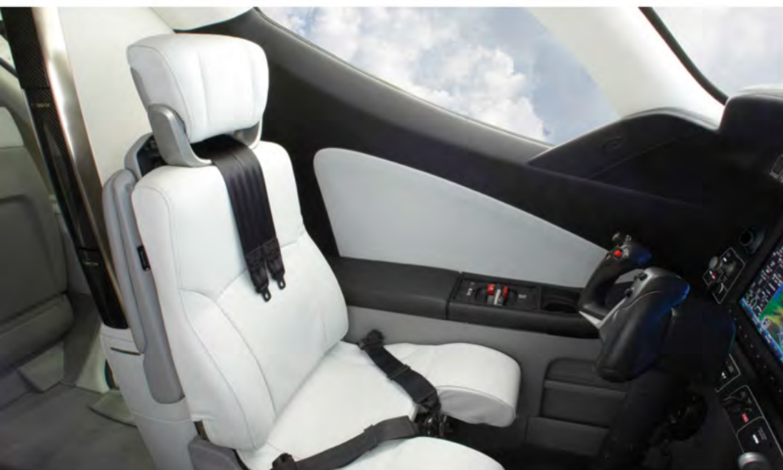
Single- or two-pilot operation of the HondaJet from its spacious, comfortable, functional crew seats—each with a retractable armrest
