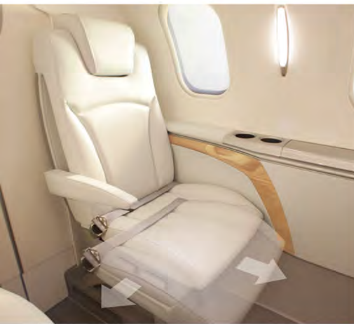
Multi-axis seats slide, shift and lock without the restraint of a track*
