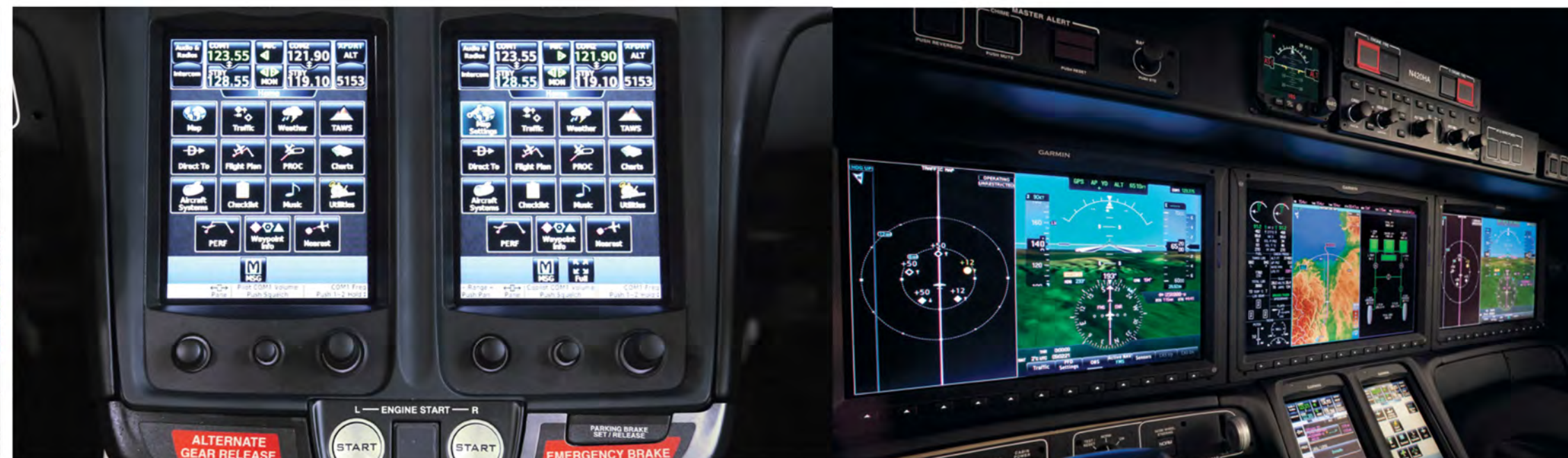
More control at the pilot's fingertips with the dual-glass touchscreen controller on the Garmin G3000 and racecar-inspired start buttons
