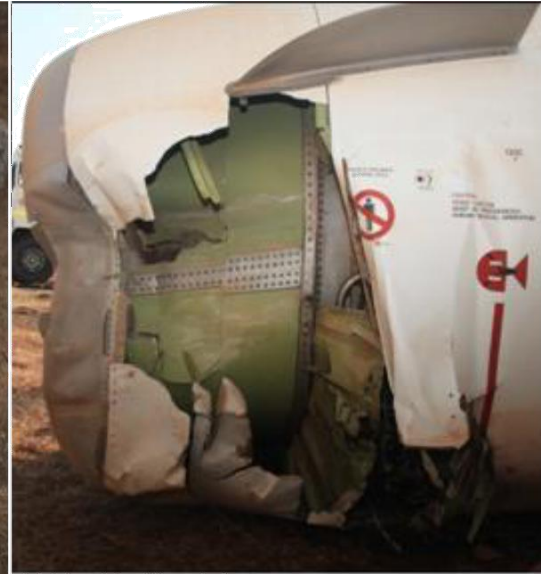
Engine damaged due hitting pillar
