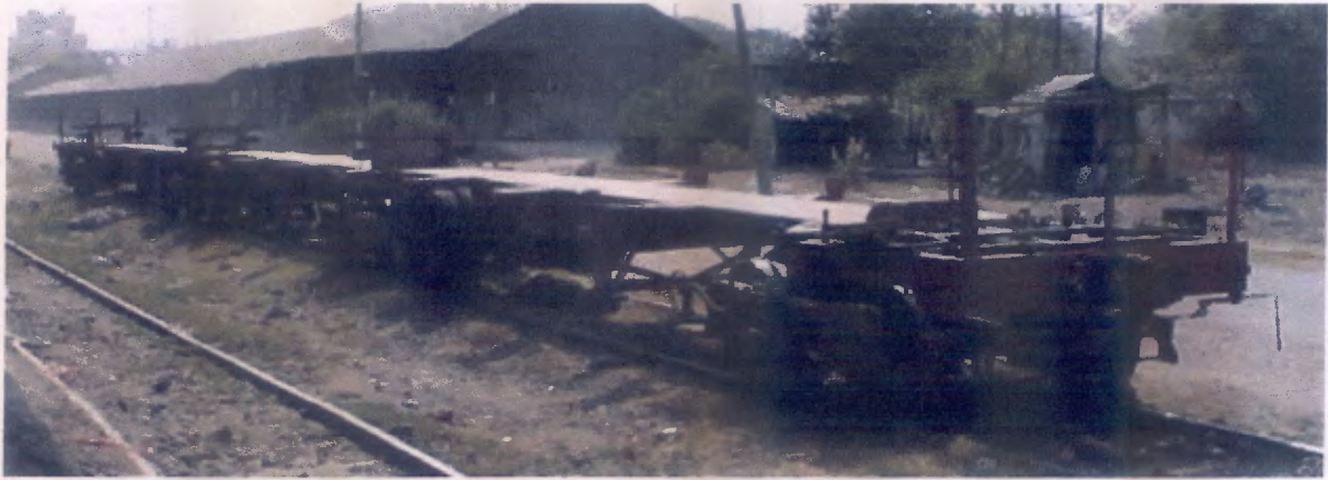
RoadRailer Prototype Rake with Tyres shown lifted clear off the Rails
