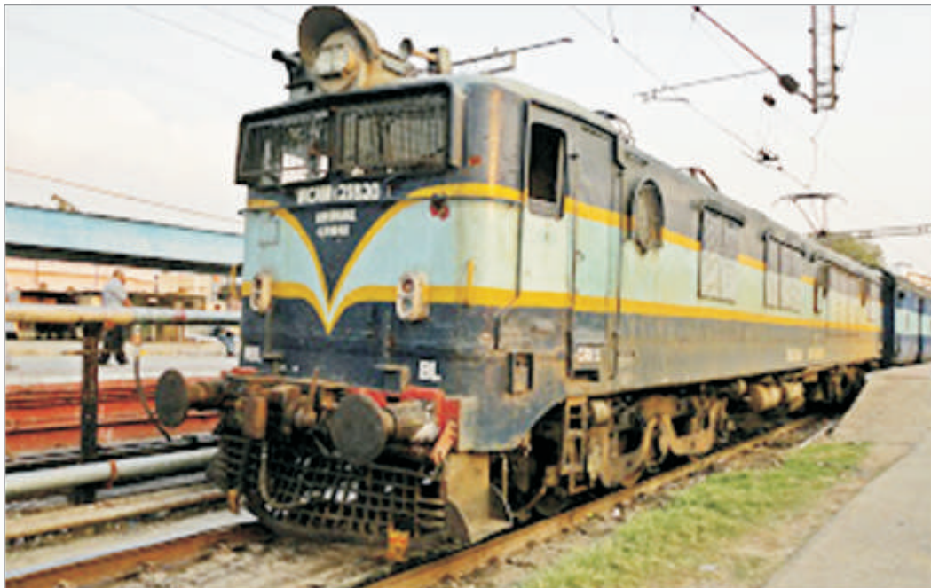
WCAM 1 (AC/DC) - Introduced in 1975 having hp of 2930 DC/3640 AC & max. speed 110 kmph. This class of loco was generally found only in Bombay Central - Ahmedabad section.
