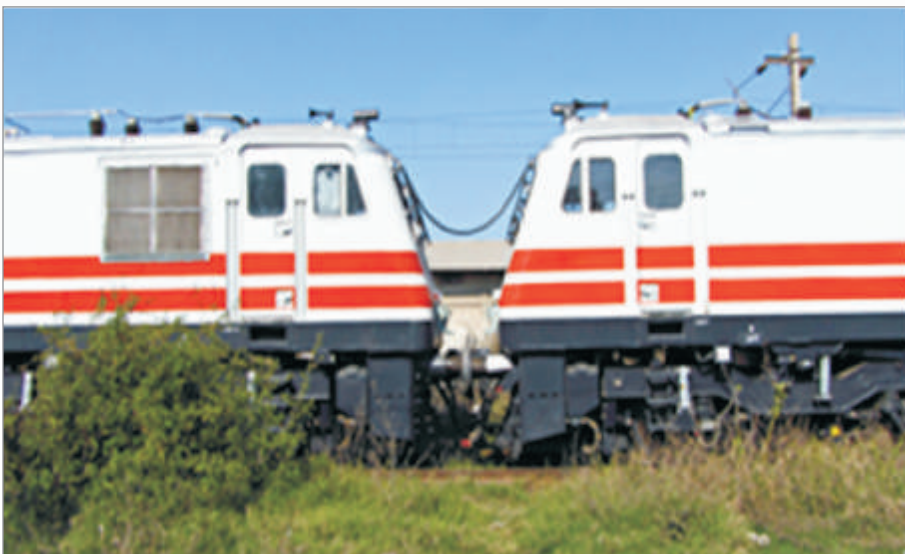
WAP 5 MU with Power through HV Cable
