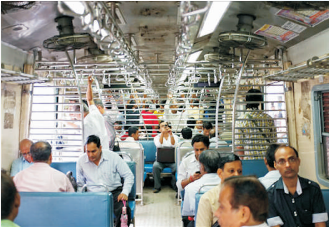
EMU fitted with LED lighting
