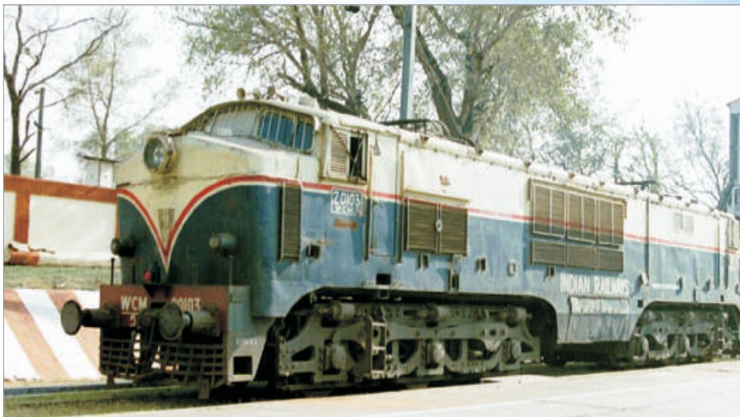
WCM 1 (DC) - Manufactured by English Electric/Vulcan Foundry. First electric loco of 3700 hp with speed potential of 105-110 kmph used in India.
