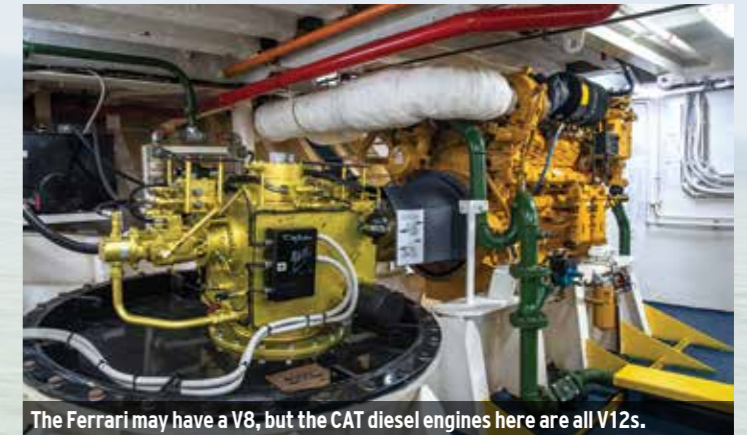
The Ferrari may have a V8, but the CAT diesel engines here are all V12s.
