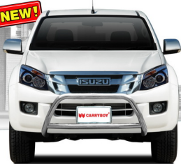
CB-765 Stainless Front Nudge Guard Manufacture a wide range of stainless steel front nudge guard for pickup/truck. Provides rugged protection on and off the road premium grade stainless steel (TP 304) tube \varnothing 3"
