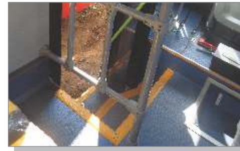
Step Well Partition
