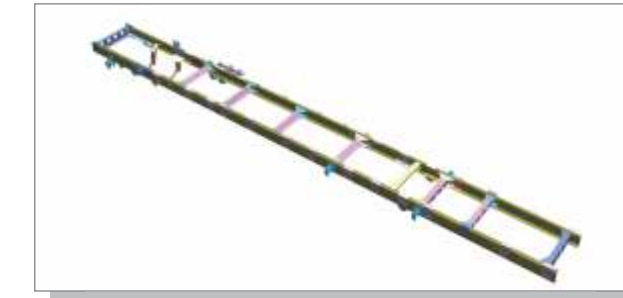
Straight Frame Chassis for Sturdier Design and Better Serviceability
