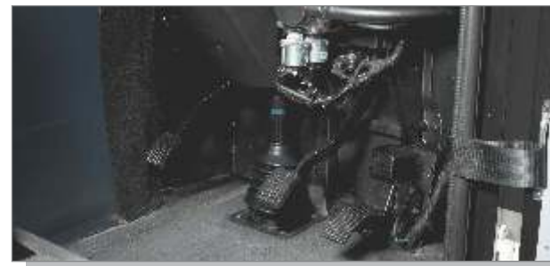
Accelerator, Brake, Clutch Efforts Reduced for Leg Comfort
