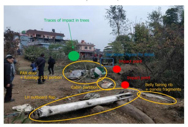
Figure 13 Site A- Identified impact points and parts
