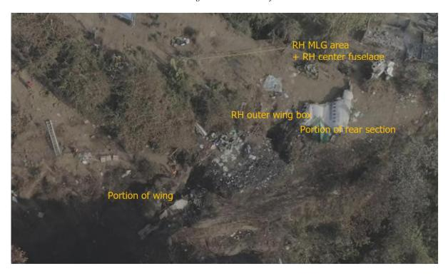
Figure 16 Blown up aerial view of components in Site B
