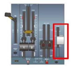
Fig: 27 location of flap lever (Source-ATR)
