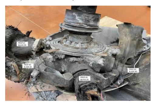
Figure 25 Prop #1 hub assembly
