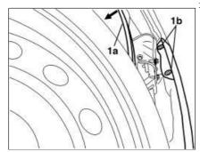
1. Move the wheel arches (1a) slightly and undo the side bolts (1b) fixing the bumper.
