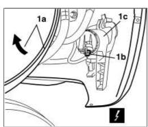
1. Move the wheel arch (1a) slightly and disconnect the electrical connection (1b) for the fog lights (1c).
