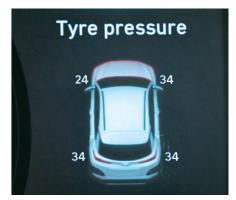
Tyre Pressure Monitoring System (High Line)
