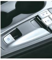
Shift-by-wire Automatic Transmission and Electiric Parking Brake
