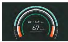
Smart eco pedal guide-encourages fuel efficient driving
