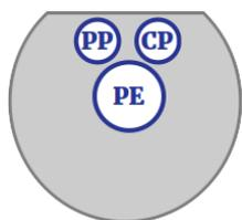
Basic signalling (BS) is used for safety-related functions, indicating for example if the connector is plugged in, before contacts are made live (or energized) and if both charging station and electric vehicle are ready for charging. Communication takes place over the signalling pins **Proximity Pilot (PP)** & **Control Pilot (CP)** between the charger, cable, and vehicle to ensure that the highest common denominator of voltage and current is selected.
