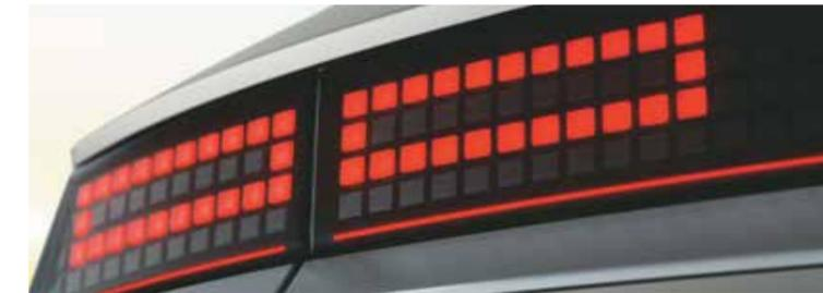
Parametric pixel LED taillamps
