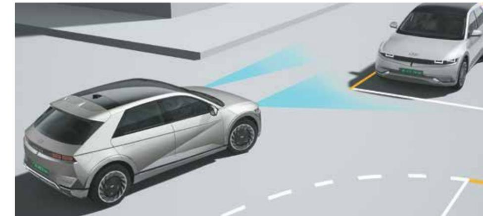
Forward collision - avoidance assist - junction turning (FCA-JT)
