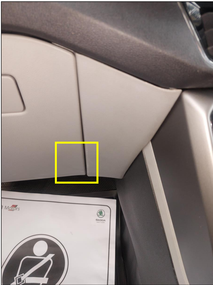
Damage to part outside glove box resembling damages due to bad usage of tools.
