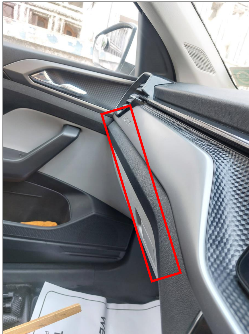
Multiple hard-pressed points resembling bad handling and placement post dis-assembly.
