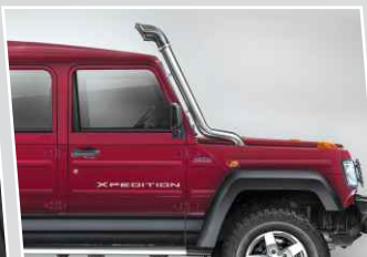
Snorkel Intake - Breathes High Altitude Fresh Air
