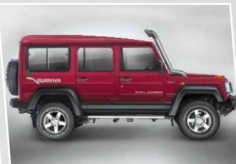
Snorkel Intake - Breathes High Altitude Fresh Air
