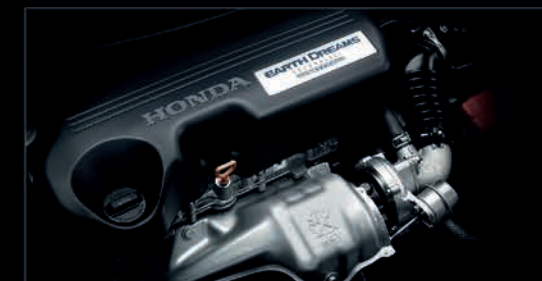
i-DTEC Diesel Engine with 6-speed MT 1.5L | 100 ps 21.9 km/l
