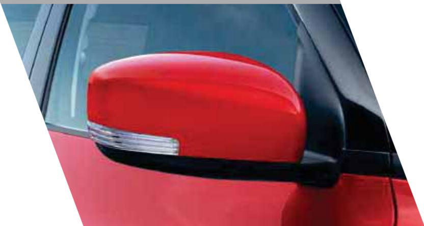
Electrically Foldable and Adjustable ORVMs with Turn Indicators
