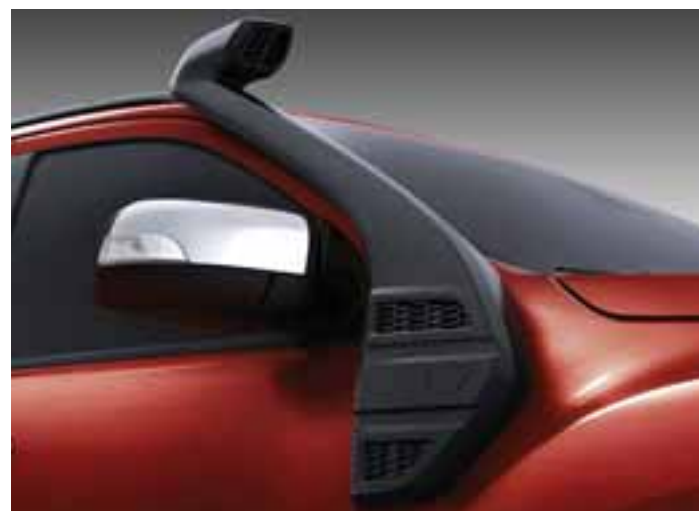
Snorkel. Draws air from roof level providing cooler cleaner air to the engine and also provides a higher air intake position to assist with water crossings.
