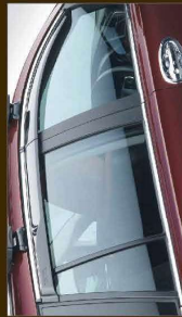
▶ Side Visor with Chrome allows you to keep the window slightly open when it's raining
