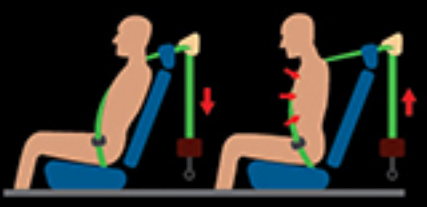
Front Seat Belt with Pre-tensioner and Load Limiters
