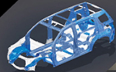
High Tensile Steel Body Construction with Tailor-welded Blanks and Side Anti-intrusion Bars
