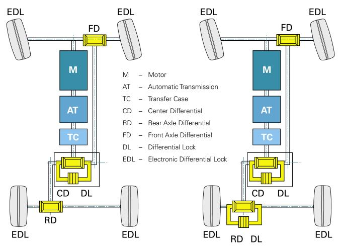
The adjustable multi-plate clutch of the center differential is automatically controlled by the Differential Control Module J646.
