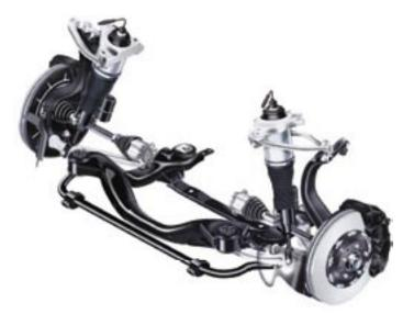
Harshness occurs when a vehicle vibrates from moving across road joints, projections, stepped differences, or depressions on paved roads. Driving on the expressway increases the pitch of the thumping sound. The impact force from the road surface causes the tires to vibrate. The tires transmit the vibration through the suspension system to the car body. Harshness has a frequency of 30 to 60 Hz.
