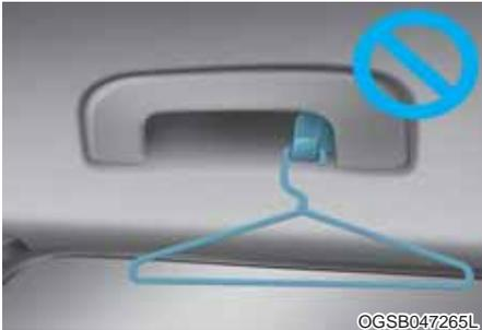
Do not hang other objects such as hangers or hard objects except clothes. Also, do not put heavy, sharp or breakable objects in the clothes pockets. In an accident or when the curtain air bag is inflated, it may cause vehicle damage or personal injury.
