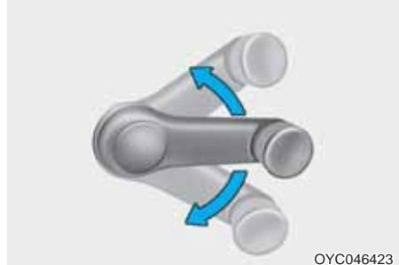
To raise or lower the window, turn the window regulator handle clockwise or counterclockwise in right side. And left side is opposite direction.
