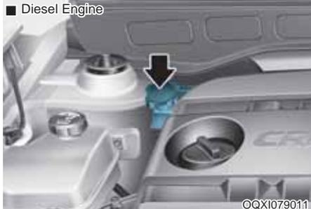
Check the fluid level in the reservoir periodically. The fluid level should be between MAX (Maximum) and MIN (Minimum) marks on the side of the reservoir.
