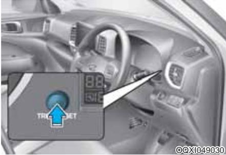
The trip computer is a microcomputer-controlled driver information system that displays information related to driving, when the ignition switch is in the ON position. All stored driving information (except odometer) resets if the battery is disconnected.
