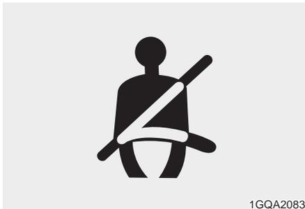
As a reminder to the driver the driver's seat belt warning lights will illuminate for approximately 6 seconds each time you turn the ignition switch ON regardless of belt fastening.
