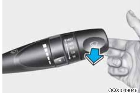
In the OFF position, pull the lever gently toward you to spray washer fluid on the windshield and to run the wipers 1-3 cycles. Use this function when the windshield is dirty. The spray and wiper operation will continue until you release the lever.
