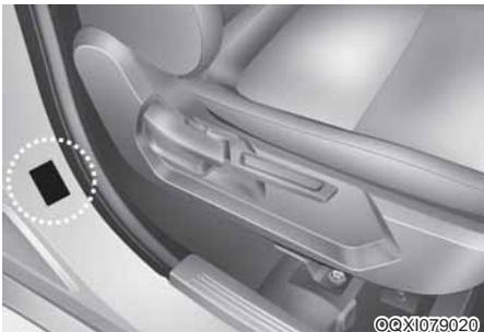
All specifications (sizes and pressures) can be found on a label attached to the vehicle.
