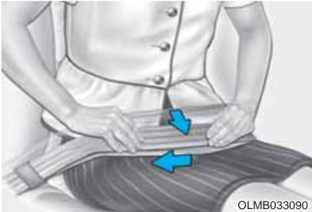
With a 2-point static type seat belt, the length must be adjusted manually so it fits snugly around your body. Fasten the belt and pull on the loose end to tighten. The belt should be placed as low as possible on your hips, not on your waist. If the belt is too high, it could increase the possibility of your being injured in an accident.
