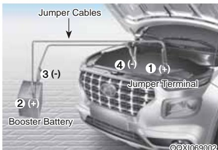
4. Connect the jumper cables in the exact sequence shown in the illustration. First connect one jumper cable to the red, positive (+) jumper terminal of your vehicle (1).
