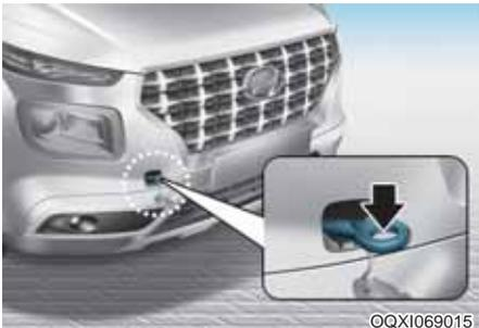
1. Open the tailgate, and remove the towing hook from the tool case.
