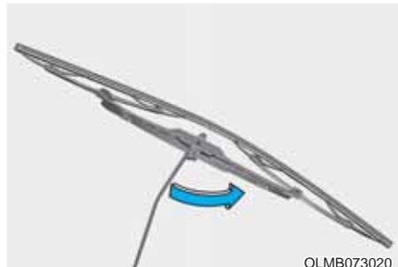
1. Raise the wiper arm and turn the wiper blade assembly to expose the plastic locking clip.
