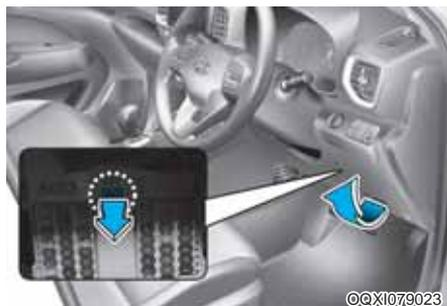
Your vehicle is equipped with the memory fuse to prevent battery discharge if your vehicle is parked without being operated for prolonged periods. Use the following procedures before parking the vehicle for prolonged periods.
