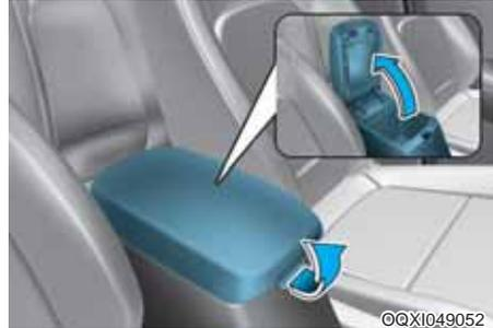
To open the center console storage, pull up the lever.
