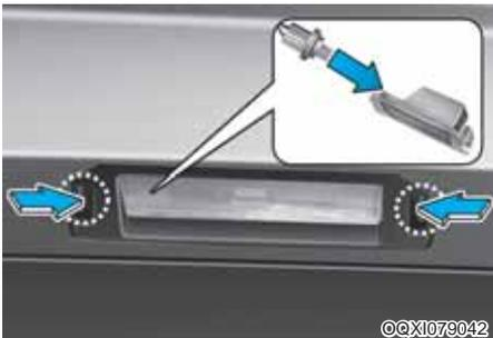
1. Using a flat-blade screwdriver, remove the light assembly from the body of the vehicle by prying the housing and pulling the assembly out.
