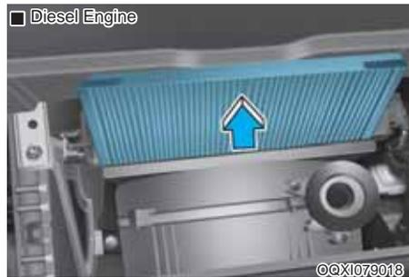
3. Remove the climate control air filter cover by pushing or pressing the clip (1) on left side.
