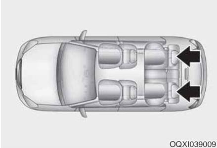
The rear seats are equipped with headrests in all the seating positions for the occupant's safety and comfort. The headrest not only provides comfort for passengers, but also helps to protect the head and neck in the event of a collision.
