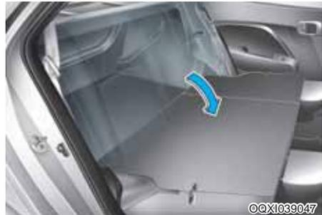
4. Pull up both sides of the seatback lever and fold the seatback toward the front of the vehicle.
