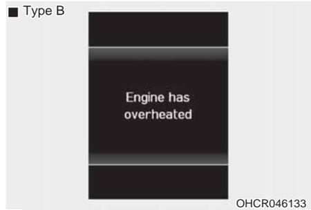
This warning message illuminates with a warning chime when the engine coolant temperature is above 120°C (248°F). This means that the engine is overheated and may be damaged.
