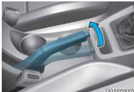
Check the stroke of the parking brake by counting the number of “clicks” heard while fully applying it from the released position. Also, the parking brake alone should securely hold the vehicle on a fairly steep grade. If the stroke is more or less than specified, we recommend that the system be inspected by an authorized HYUNDAI dealer.
