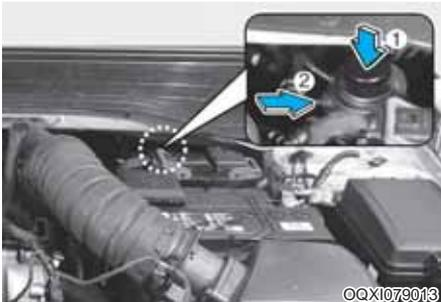
If you drive until you have no fuel left or if you replace the fuel filter, be sure to extract air from the fuel system as it makes it difficult to start the engine.
