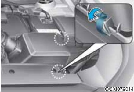
You can clean the filter when inspecting the air cleaner element.
