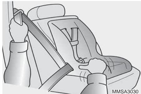
3. Buckle the seat belt and allow the seat belt to take up any slack. After installation of the child restraint system, try to move it in all directions to be sure the child restraint system is securely installed.
