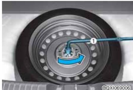
If it is hard to loosen the tire hold-down wing bolt by hand, you can loosen it easily using the wheel lug nut wrench.
