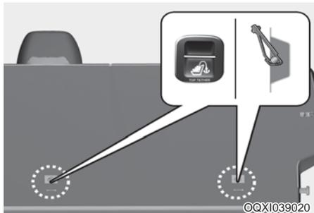
First secure the Child Restraint System with the ISOFIX anchorages or the seat belt. If the Child Restraint System manufacturer recommends the top-tether to be attached, attach and tighten the top-tether to the top-tether anchorage. Top-tether anchorages are located on the back of the rear seats.
