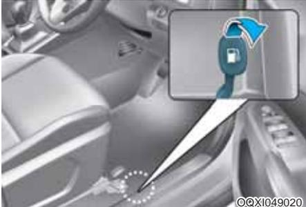
The fuel filler door must be opened from inside the vehicle by pulling up the fuel filler door opener.
