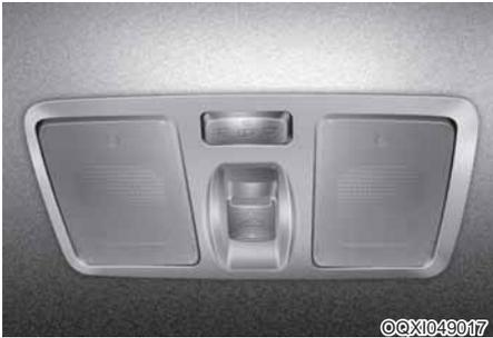
If your vehicle is equipped with a sunroof, you can slide or tilt your sunroof with the sunroof control switch located on the overhead console.
