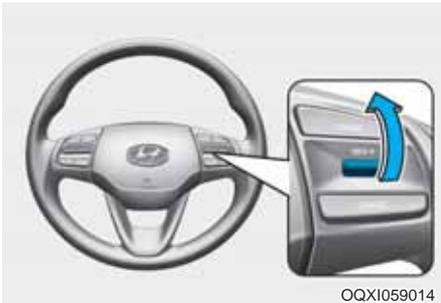
Push the toggle switch up (RES+). If the vehicle speed is over 30 km/h (20 mph), the vehicle will resume the pre-set speed.
