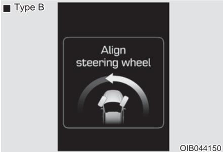
This warning message illuminates if you start the engine when the steering wheel is turned 90 degrees to the left or right.
