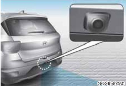
The Rear View Camera will activate when the ignition switch is in the ON position and the shift lever is in the R (Reverse) position.
