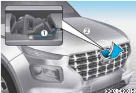
3. Go to the front of the vehicle, raise the hood slightly, push the secondary latch up (1) inside of the hood center and lift the hood (2).
