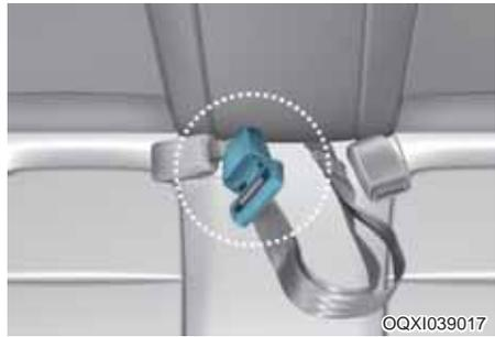
When using the rear center seat belt, the buckle with the “ENTER” mark must be used.
