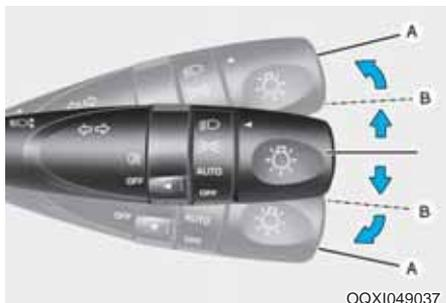
To signal a turn, push down on the lever for a right turn or up for a left turn in position (A). To signal a lane change, move the turn signal lever slightly and hold it in position (B). The lever will return to the OFF position when released or when the turn is completed.
