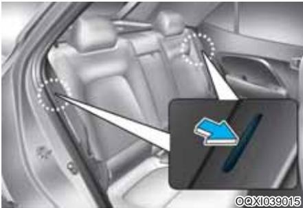
3. Insert the rear lap/shoulder belt plate into the holder on the side trim. It will prevent the lap/shoulder belt from interfering with the seatback when folding.
