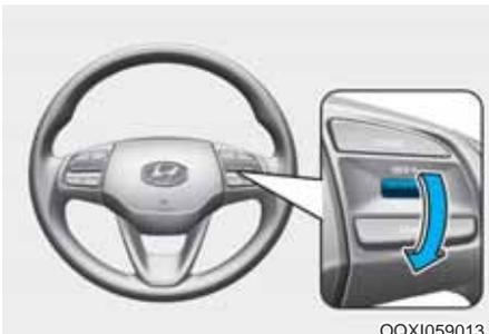
3. Push the toggle switch down (SET-), and release it. The SET indicator or set speed on the LCD display will illuminate.
