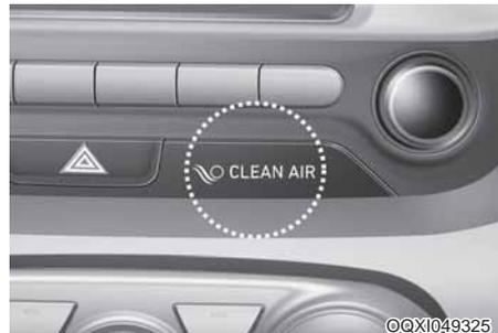
When the ignition switch is in the ON position, the clean air function turns on automatically.
