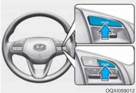
1. Press the CRUISE button on the steering wheel to turn the system on. The cruise indicator will illuminate.
