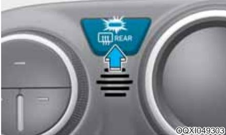
The defroster heats the window to remove frost, fog and thin ice from the interior and exterior of the rear window, while engine is running.
