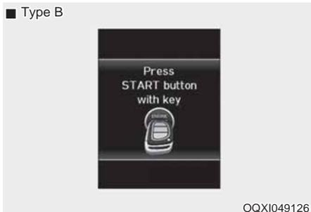
This warning message illuminates if you press the Engine Start/Stop button while the warning message “Key not detected” is illuminated.
