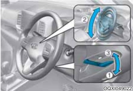
Pull down the lock-release lever (1) on the steering wheel column and adjust the steering wheel angle (2). Move the steering wheel, so it points toward your chest, not toward your face. Make sure you can see the instrument panel warning lights and gauges.
