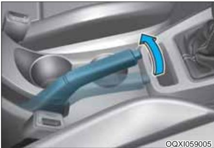
Always set the parking brake before leaving the vehicle, to apply:
