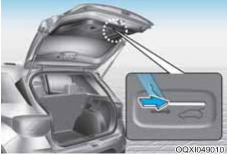
Your vehicle is equipped with the emergency tailgate safety release lever located on the bottom of the tailgate. When someone is inadvertently locked in the luggage compartment, the tailgate can be opened by doing as follows:
