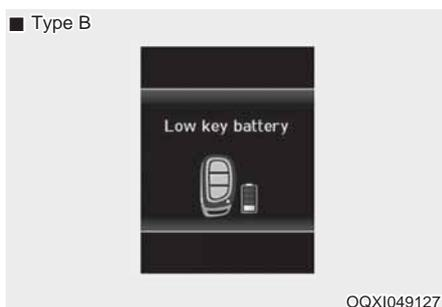
This warning message illuminates if the battery of the smart key is discharged when the Engine Start/Stop button is in the OFF position.
