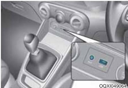
You can use a USB port to plug in a USB or an iPod®.
