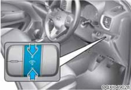
The brightness of the instrument panel illumination changes by pressing the upper or lower part of the switch when the ignition switch is in the ON position and when the parking lights are turned on.
