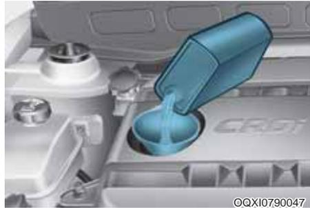
If it is near or at L (Low), add enough oil to bring the level to F (Full). **Do not overfill.**
