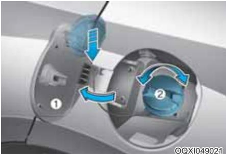
3. Pull the fuel filler door out (1) to fully open.
