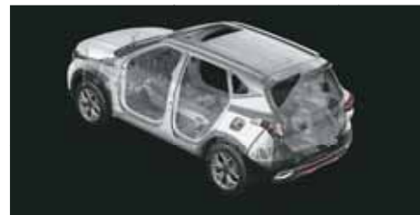
73% HIGH STRENGTH STEEL STRUCTURE Kia Seltos structure uses High-strength steel and adhesives for comprehensive safety.
