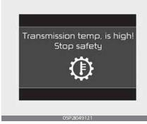
Under certain conditions, such as repeated stop-and-go launches on steep grades, sudden take off or acceleration, or other harsh driving conditions, the transmission clutch temperatures will increase excessively. Finally the clutch in transmission could be overheated. 6
