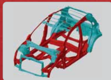
G-CON body disperses and absorbs collision impact
