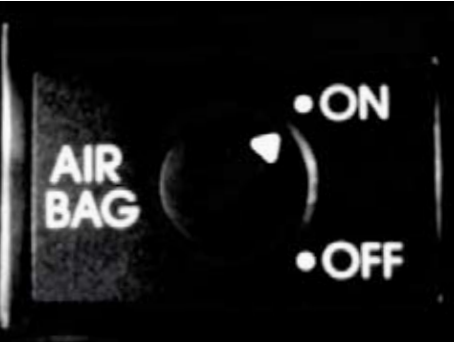
The front passenger's airbag can easily be deactivated with the key of the vehicle.
