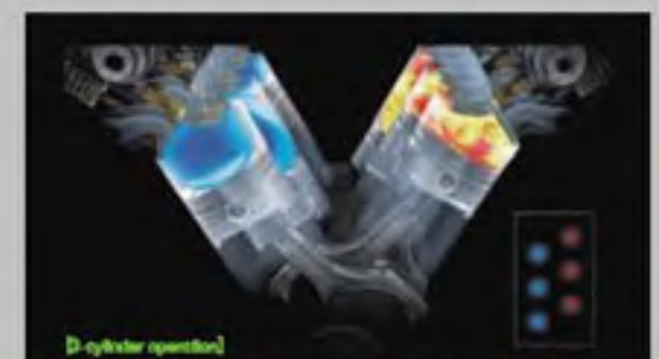
At low cruising speeds and with low engine loads, it runs on just 3 cylinders.
