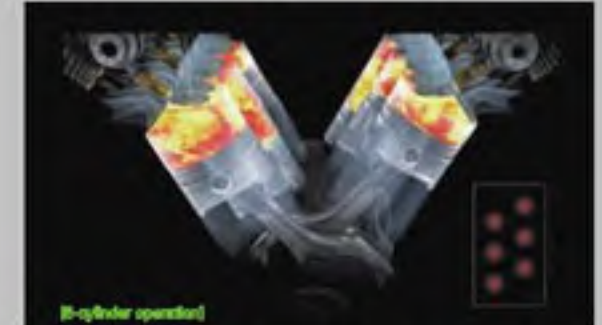
All 6 cylinders in use while starting up, accelerating or going up.
