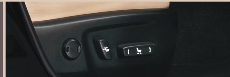
10 Way Adjustable Power Driver Seat with Lumbar Support
