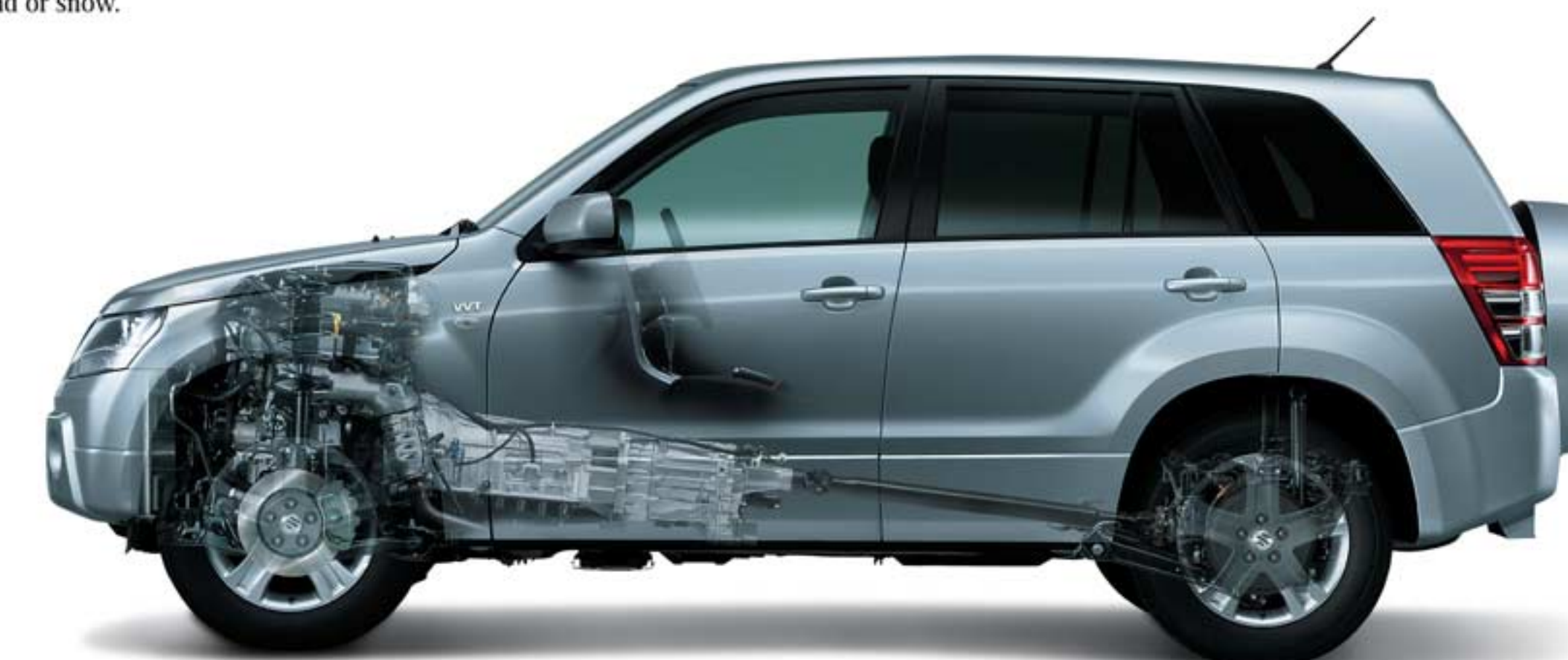
4 Low Lock: Central differential locked. Power sent to front and rear wheels equally but after increasing the torque using a 'traction enhancer'. Switch to this mode when stuck in mud, sand or snow.
