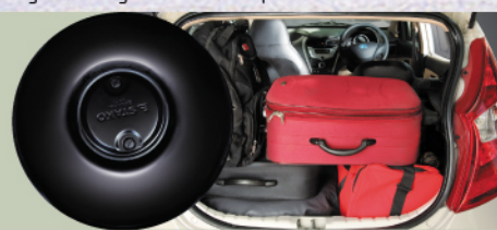
Tank capacity (water filling) - 34 litres
