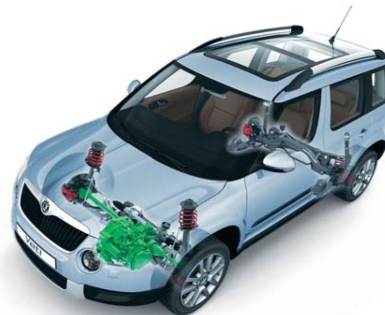
Škoda Yeti with a front-wheel drive (1.2 TSI/77kW and 2.0 TDI CR DPF/81kW engines)
