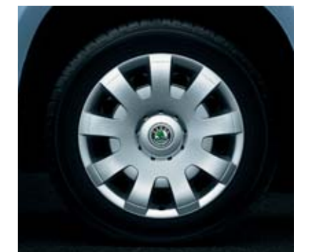
7.0J x 16" steel wheels for 215/60 R16 tyres with Rif hub covers.
