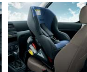
ISOFIX G 0/1 child seat (5L0 019 905, 5L0 019 905A-E) with RWF frame for rear-facing fitting (5L0 019 902A)
