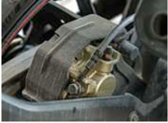
● A plastic shield keeps dirt and debris off the rear brake caliper.
