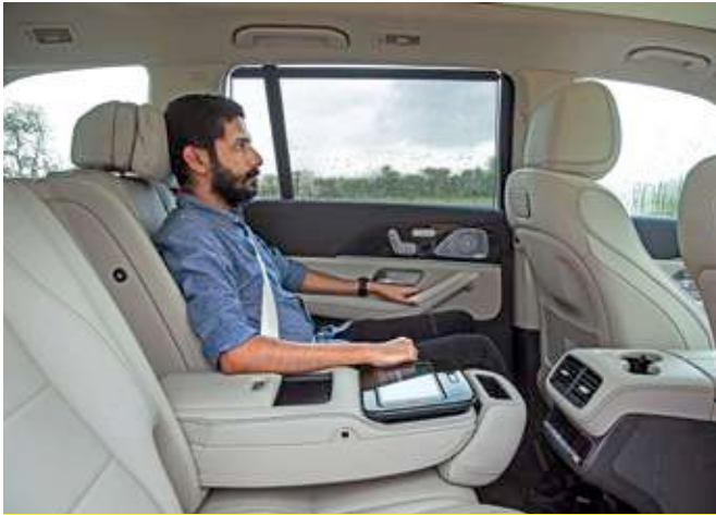
Seat slides by 100mm for superb legroom; eats into third row though.
