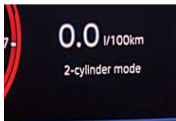
Cylinder shut-off under light load and engine stop-start lower fuel consumption.
