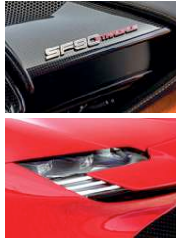
Carbonfibre abounds; SF90 is first Ferrari to use matrix LED headlights.
