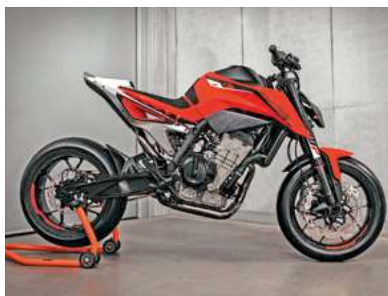
The parallel-twin will share its design with the 790 and 890 engines.
