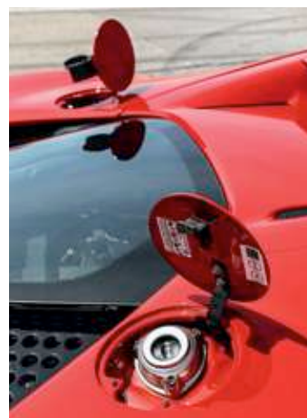
Digital dash is complex; RAC-e is on display; one for petrol, one for electricity.
