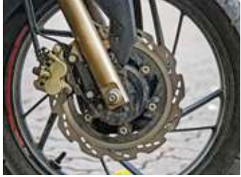
● Braking is adequate, but a larger disc would improve the performance.
