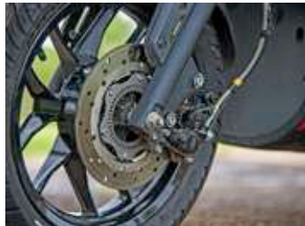
• ABS-equipped 220mm disc brake offers excellent stopping power.
