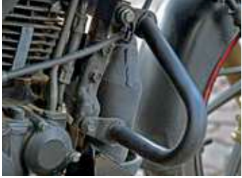
● BS6 update has added a bulky catcon on the header pipe.
