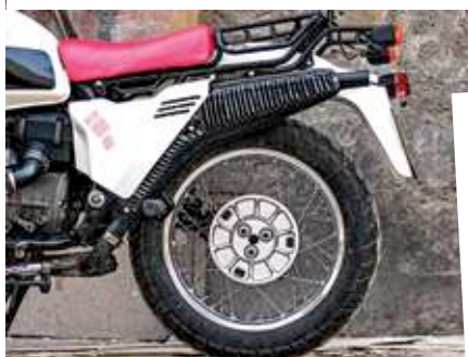
Original R 80 G/S used a rear drum brake.
