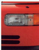
Integral flaglamps and indicators are recessed to improve aerodynamics.
