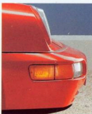
The deformable body panels encase resilient bumpers.
