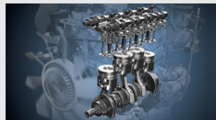
Diamond-like Carbon-coated Pistons and Injectors
