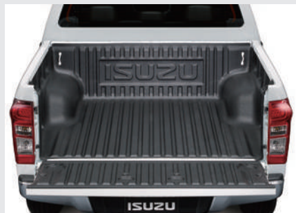
Bed Liner Under Rail
