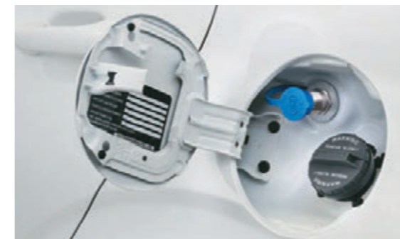
Convenient CNG filling valve location near petrol fill area
