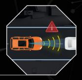
Adaptive Cruise Control is an advanced version of cruise control. It senses and monitors the road ahead and automatically accelerates/decelerates for maintaining a proper distance from the vehicle in front.
