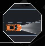
Intelligent Headlamp Control activates and deactivates the high-beam, depending on the oncoming traffic and environment situation. Thus preventing other road users from blinding due to high-beam.
