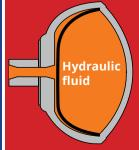
When the diaphragm leaks it will allow the gas out and fluid will fill the sphere making the suspension solid.
