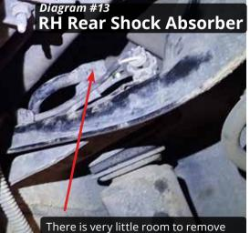
There is very little room to remove hydraulic line bracket and the shocker nut, but it can be done.
