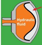
When in good condition, the gas sealed by the diaphragm acts as a spring and the force is transferred by the hydraulic fluid.
