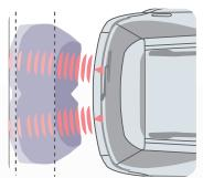
• Sense every obstacle in the rear with the **back sonar** while reversing or parking.
