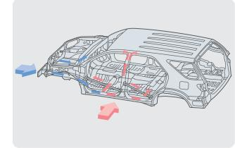
The sturdy GOA (Global Outstanding Assessment) body lessens the impact of a front or side collision and adds to the toughness of the cabin.
