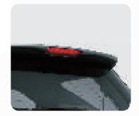
A thin 6-LED type high-mount stop lamp gives a classy appearance. It also makes the car visible from a far distance at night.
