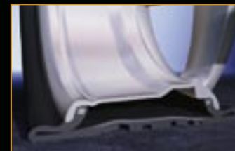
Conventional tyres when all pressure is lost: tyre is destroyed within a short distance.
