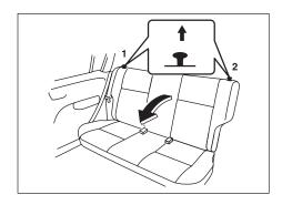
Fold the rear seat by pulling the knob 1 and 2 together as shown, in order to access the spare wheel.
