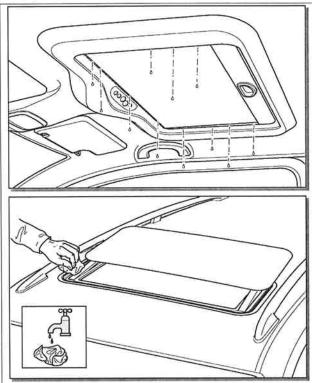
Check seal when sunroof leaks. Clean seal with a wet cloth. Apply talcum powder.
