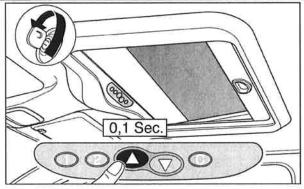
For preventing roof from closing automatically, press ▲-button briefly within 3 seconds after switching off ignition.
