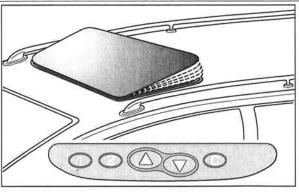
By pressing button  $\triangle$  or  $\nabla$  continuously, panel is adjustable in 4 different positions. When button is released, roof remains in momentary position.
