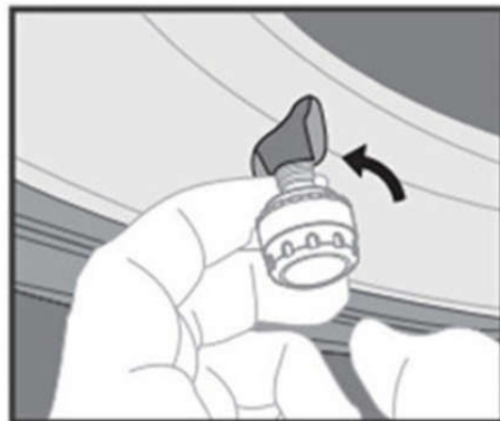
C Screw anti-thief nut by anticlockwise to fix sensor
