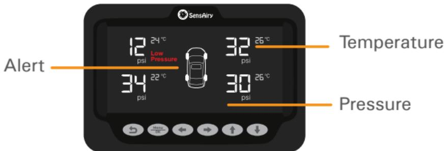
Tyre Pressure data is shown in bigger number in units of psi. Maximum pressure that can be displayed is 99 psi and minimum is 0 psi. Next to tyre pressure, tyre temperature is shown as superscript in units of Celsius. Maximum temperature displayed is 99°C and minimum is -40°C.
